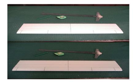
64. Bond the outer wing panels to the wing center section. Hold together with tape, allow the bond to cure with the wing flat on the table; top side down. Note: The wing panels might be slightly different in size compared to the center section. Nothing is perfect, it's easy to fix, for now match the upper surfaces.
