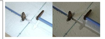
80. Test fit the torque rod assemblies in the slot for freedom of movement, ¾ inch from one extreme to the other is enough.
