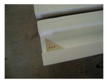
3. Use the nose gear hardware to locate the nose gear wheel well, then cut the well out. Make the well slightly oversized and angled to allow air to pass through the nose wheel well for battery cooling.
