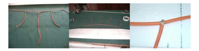
72. Strip the wire at the marks made while it was in the wing. Soldier the 9 inch sections to the outside striped sections and what's left goes on the striped section at the center. Repeat this step for the other section of wire in slot #1.
