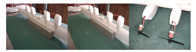
107. Solder the motors to the leads hanging out of the nacelles. Be careful with the soldering iron. Just a touch will ruin the foam. Put the motors in the nacelles giving them a twist as they go in. Test run the motors to check that they all turn the proper direction. Use two "d" cells; do not use the flight pack. It will fly right off the table.
