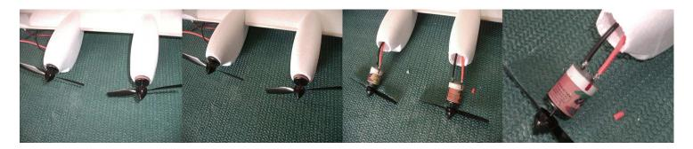
108. Pull the motors out until the tape shows then cote the motors sides with silicone all the way around. Then push them in as you did before. Wipe off the excess silicone
