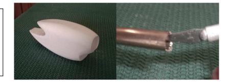
102. Sand the corners off the engine nacelles. Keep an eye on the area around the circle that makes the motor mount so you don't sand it too thin. Test fit the nose cone frequently. You are looking for a snug fit.
