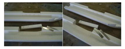
2. Epoxy the nose gear braces (NGB) 34 inch aft of the front of the fuselage. We have included a nose gear assembly supplement to cover the assy of the tandem nose wheel in more detail.
