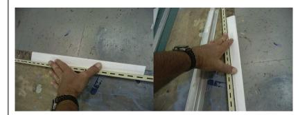
83. With the wing flat on the table transfer the aileron centerline to the wing. Use a highlighter pen and lightly run it down the "point" on the "V" you sanded on the aileron. Quickly, before it dries, press it against the wing with both parts flat on the table.
