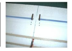
79. Place the completed torque rod assemblies on slot #3 with one of the arms over the marks made ½ inch off the centerline. Mark location of the arm at the other end, and then remove the torque rods. Use the hot wire to melt clearance slots for the arms. Use caution at the outboard slots not to go through the wing, work slowly with a cooler wire than before.
