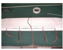
74. Lay the harnesses in their slots. Note: the wires at the centerline point toward each other.
