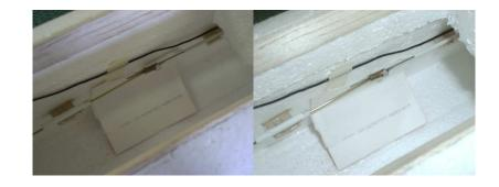
62. Epoxy the back door in place and hold with tape until it cures. Sand flush, tape the nose cone off and paint with primer. This will ensure that foam safe paint will stick to the plastic nose cone.
