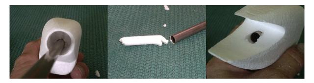
103. Use tweezers, needle nose pliers, or forceps to pick out the foam from the pre-cut "motor mount hole". It's about 3 inches deep. Next use your ½ inch razor hole saw to cut a hole at the bottom of the motor mount hole. Cut all the way through. It should come out where the engine nacelle contacts the bottom of the wing and centered. Keep going to form a slot for the wire about 2 inches. Note you will need a stick to clear the saw hole of debris.
