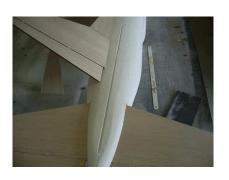
35. Sharpen a section of clothes hanger, then align it between where the control horn will be and where it will exit the fuselage. Push it into the fuselage, aiming for the center of the fuselage until it exits the fuselage ceiling. Remove the wire, then install the control rod sheathing.
