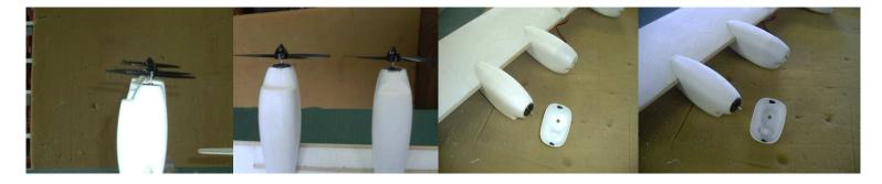
109. Check the motors for alignment by comparing the props to each other in both directions, from the side and the top. When you are happy with the alignment allow it to set up over night.
