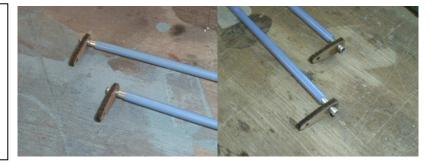
78. Sand the tips of the aluminum tubes to give CA something to bond to, then CA torque arms to one end of the tube. Slide the plastic torque rod bearing over the torque rod, then CA the other torque arm to the other end of the tube. Note: avoid getting CA into the bearing by applying the CA to the outboard portion of the arms only. A little rotation will work the CA into the joint. Also be sure that the arms are in the same position by laying them flat on the table.
